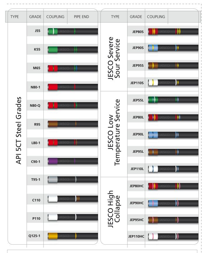
**JESCO's** proprietary steel grade color identification system is user friendly allowing our products to be easily identified. Special clearance couplings will be painted with a grey band adjacent to the color identification band on the coupling.
